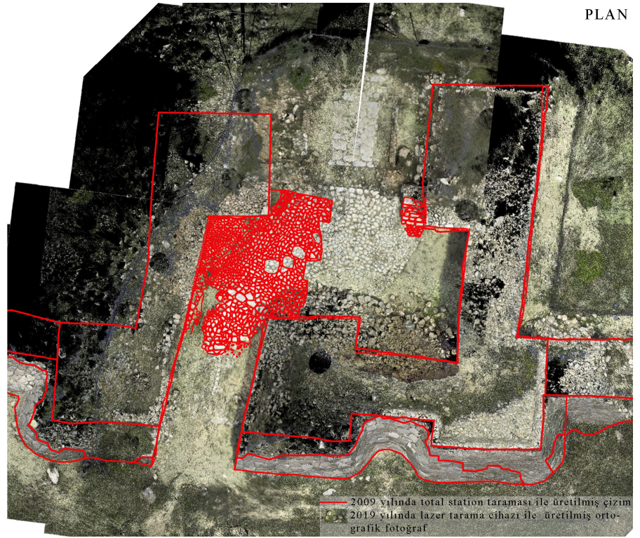
Figure 18. Cappadocia Gate: The comparison of the plan produced from the 2009 total station point cloud (in red) and the combined orthophoto produced from the 2019 ground laser scan data. The image was produced by M. Çingir Salman, Doğan Tekin and Nurçe Düzialan Salman in 2022. (Image: Kerkenes Project)
