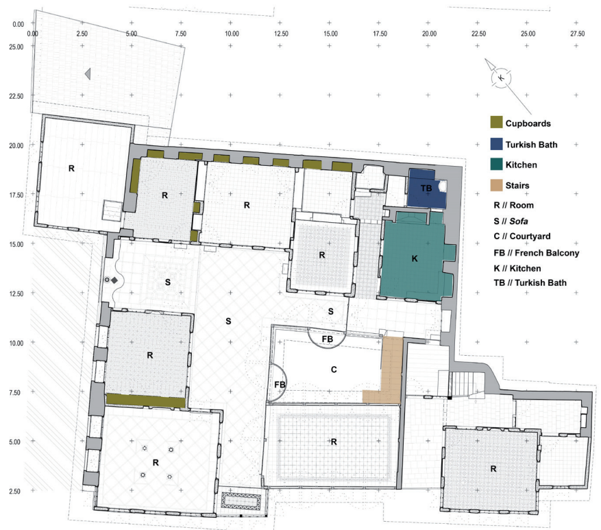
Figure 8. First-floor spatial organisation and architectural elements of traditional housing in plot 553 during the French Mandate Period (Prepared by the author, 2021).
