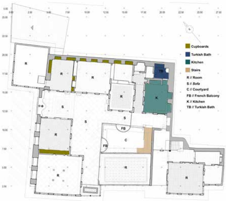
Figure 8. First-floor spatial organisation and architectural elements of traditional housing in plot 553 during the French Mandate Period (Prepared by the author, 2021).
