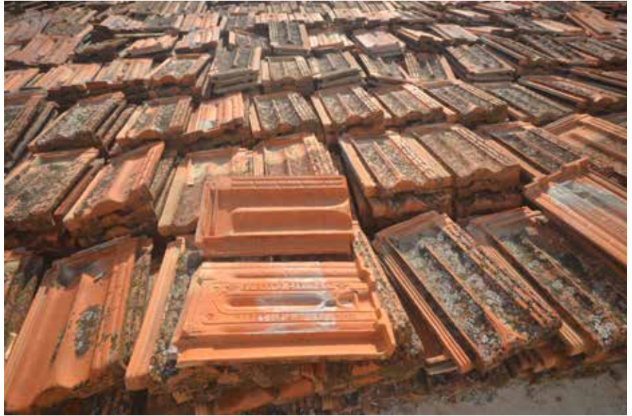
Figure 20. Guichard Carvin&Co. Marseille St. Andre-France stamped tiles with a bee logo that were used in the building (Photograph taken by the author, 2020).
