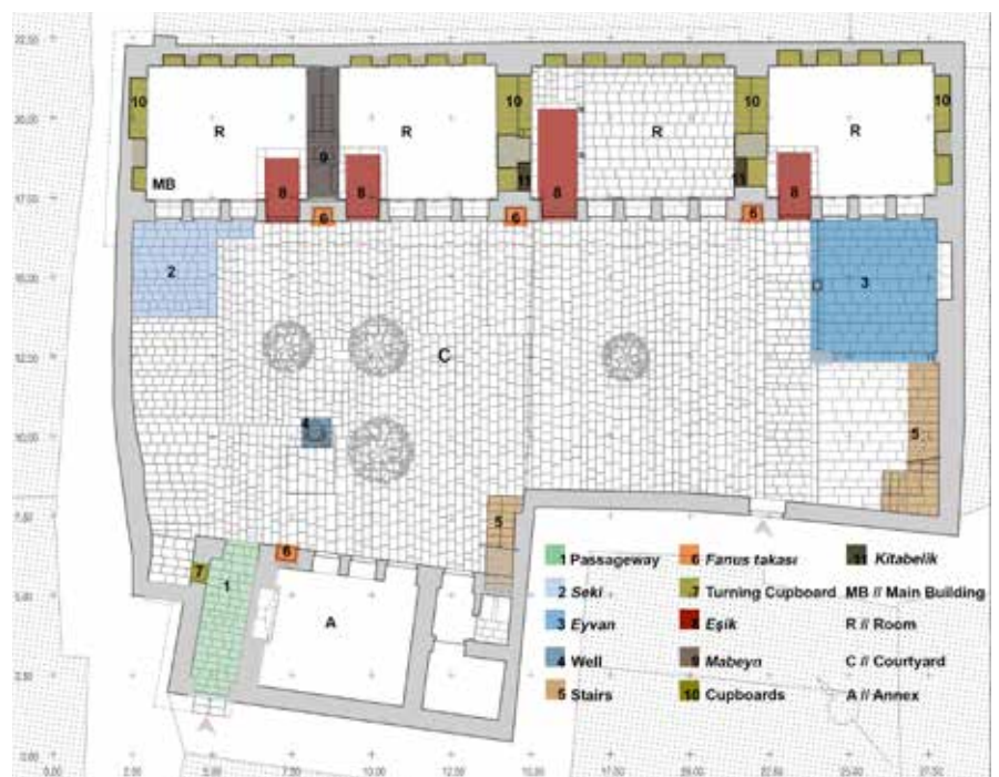
Figure 2. Typical spatial organization and architectural elements of a traditional Ottoman Period Antakya house which is located in 4 th circumscription plot number 1250 (Prepared by the author, 2021).
