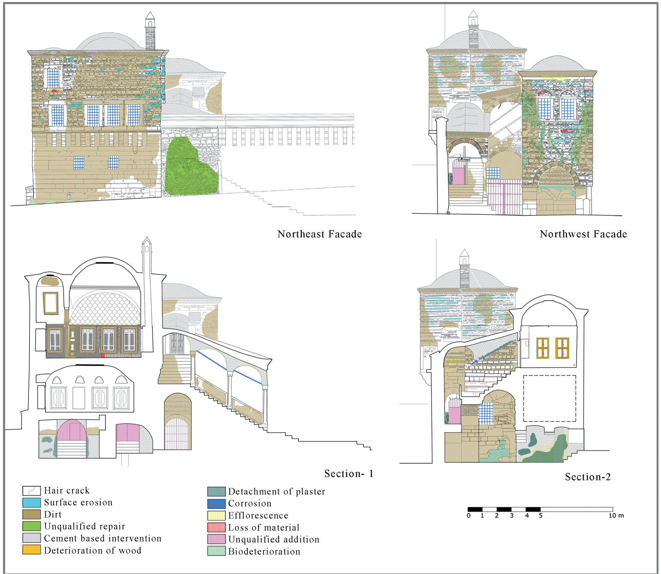
Figure 20. Samples of Deterioration Analysis, 2012.
