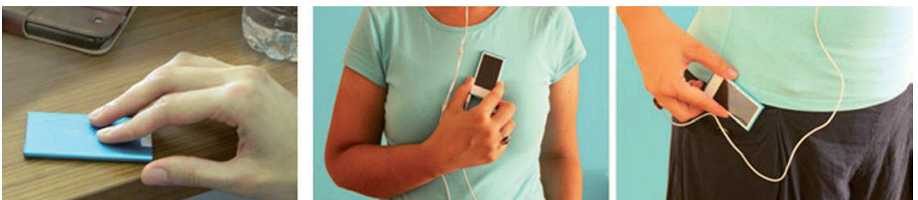
Figure 3. Pausing the song by reversing the music player, changing the place of the device to change the playlist
