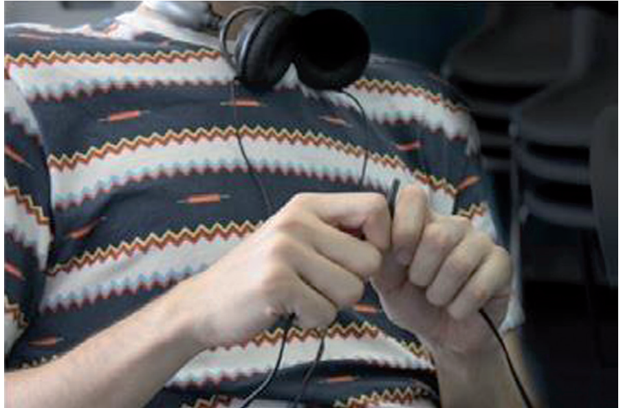
Figure 2. Decreasing volume by bending the cable
